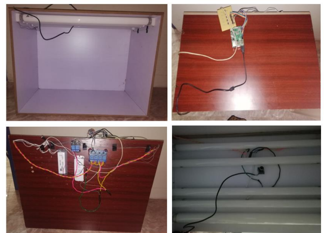
Figure 5.1 Complete hardware setup of automatic hue matching cabinet.
